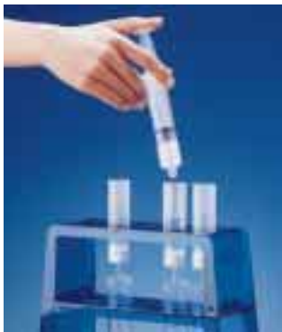
Figure 5. The QIAfilter Cartridge in use.
