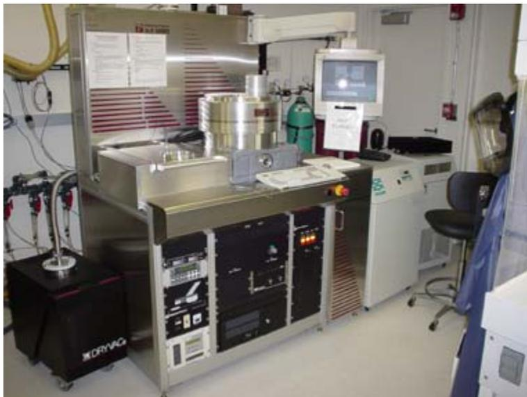
Figure 2: The Silicon Reactive Ion Etching (SiRIE) system at UCSB's Nanofabrication Facility. [5]
