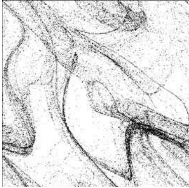
Figure 1: An example of fractal particle clustering in a numerical simulation by Bec [6]. This picture displays 10^5 particles of Stokes number 10^{-1} .
